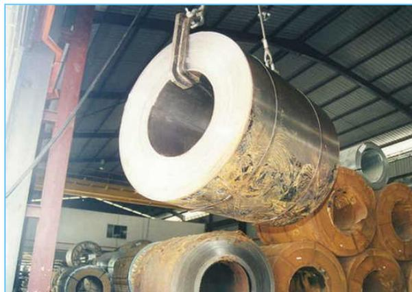
*Coils at storehouse with severe rust damage.*
